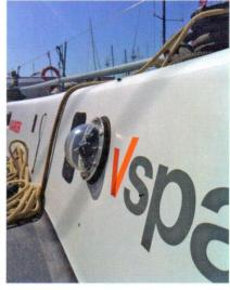
The heart of the VSpars system is a fit-PC and three cameras. Two mainsail cameras are mounted into the cockpit walls (above) while the jib/spinnaker camera is recessed into the foredeck just aft of the hatch. Each camera takes and stores a picture every 3 seconds.
